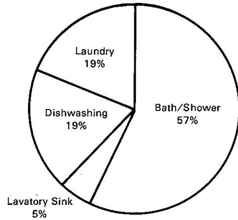
Figure IV-2. Average Residential Hot Water Use
